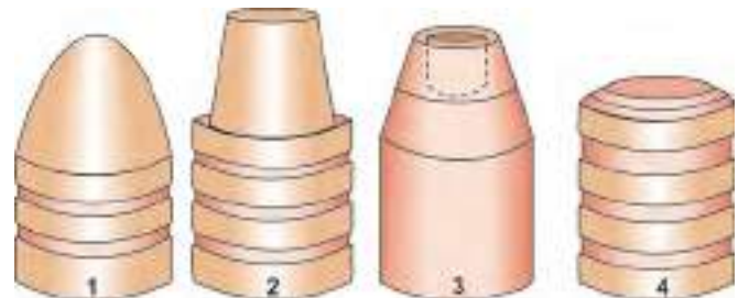
Fig. 20.1: Types of bullets presenting variety of modification: (1) Round nose, (2) Semi-wadcutter, (3) Jacketed semi-wedcutter (Hollow prints), (4) Wadcutter
