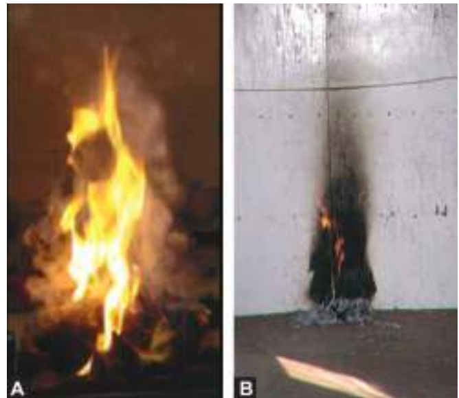
Figs 30.3A and B: An inverted “V” shaped fire pattern during and at self-extinguishment (Source: Photos courtesy of Susan Sherwin, Maricopa County Attorney’s Office)
