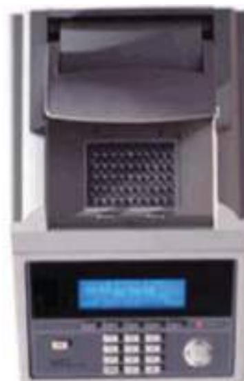
Fig. 12.6: A modern thermal cycler capable of performing 96 PCR's at a time. The model shown is ABI 9700
